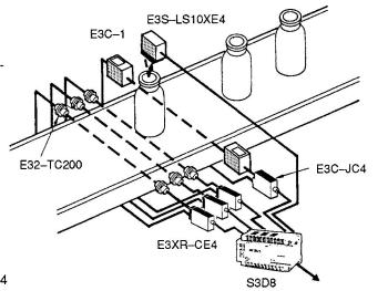
Fiber Optic Photoelectric Switch E32–TC200/E3XR Photoelectric Switch E3C–1 Limited Reflection Photoelectric Switch E3S–LS10XE4 Sensor Controller S3D8
